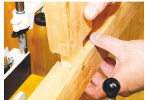
▲ The resulting mortises are clean and square
